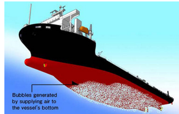
Image from the bottom of a module carrier equipped with an air lubrication system
