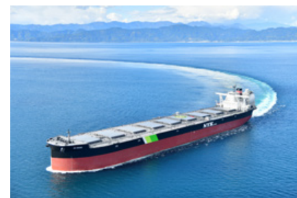
LNG-fueled capsized dry bulk carrier "SG OCEAN" (LNG dual-fuel engine-equipped ship)
