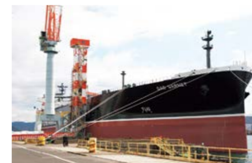
LPG carrier also able to carry ammonia "Gas Garnet" (Vessel equipped with LPG dual-fuel engine)
