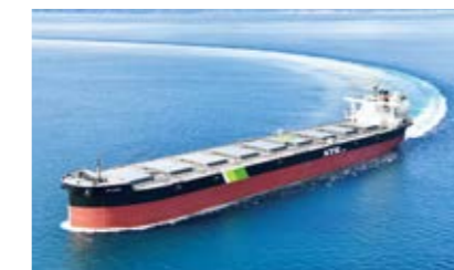
SG Ocean, an LNG-fueled capesize bulk carrier (with an LNG dual-fuel engine)
