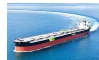
SG Ocean, an LNG-fueled capesize bulker (with an LNG dual-fuel engine)
