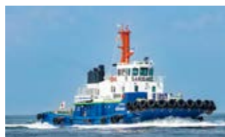
Sakigake, an ammonia-fueled tugboat which is converted from LNG-fueled tugboat
